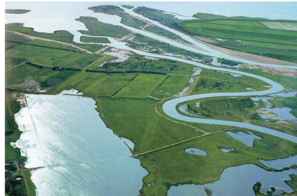
Aerial photograph of the newly 'restored' Skjern River Delta: 2.7 million m<sup>3</sup> of earth were moved and 19 km of embanked canal were converted into 26 km of meandering river. A significant part of the former meadow and wetland turned into lakes because the ground had sunken as a consequence of the drainage, 2009.
